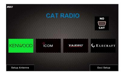
Select the desired Radio, (after connecting the Cat cable) the choice made will appear green, if we do not have a Cat connection, select the NO CAT button, pay maximum attention to the NO CAT mode, the filter must always be selected and however manually for the corresponding Band, the AUTO key cannot be selected.
