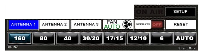
ON AIR has 3 colours to indicate different ways of PTT, BLACK colour indicates that PTT is disabled (see Operate Off-On key command), GREEN colour indicates that PTT is enabled (Operate ON), RED colour indicates you're on air.
