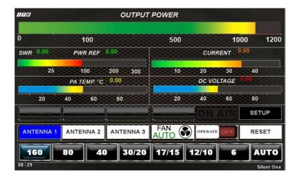
When switched on, the amplifier will automatically position itself in Band 160M and Antenna 1, (if the Cat Radio is selected, it will start in AUTO) the Fans in Automatic (FAN AUTO), and Operate Enabled (ready for PTT) (1st Ignition).
